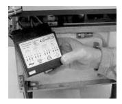
2. The connectors are very tight. To successfully remove use a crescent wrench to grip the outside of the connector rocking gently up and down while pulling up to release. The best way to work from right to left.
